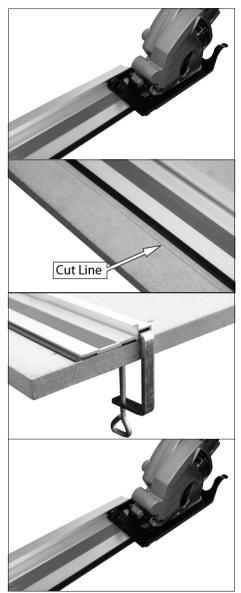
6. Release the on/off trigger and allow the saw to spring up when the saw cutting is complete.
